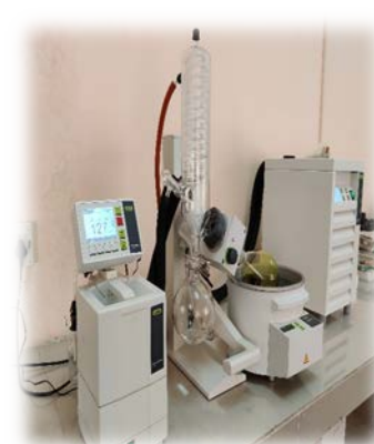
Figure 4: Drying of extract using Rotary Evaporator
